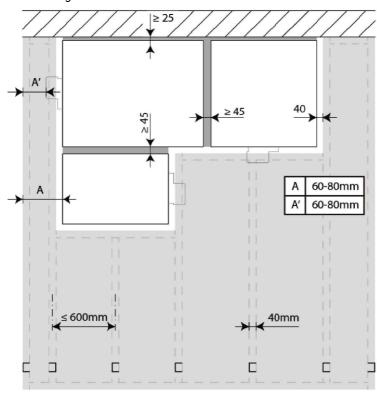
Mounting in a rigid wall at 0 distance
