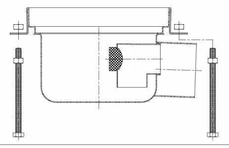
\* IN CASE APPLICATION OF ADJUSTING FEET IS REQUIRED, AS A FIRST STEP, THE BOLTS AND NUTS ARE FIXED ON THE BODY AS SHOWN BELOW.
